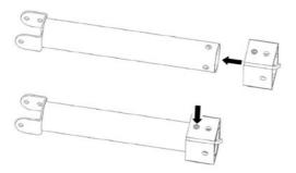
4. Attach top coupler and/or tilting mechanism to ceiling yoke. Fix to ceiling. Fix pole.
