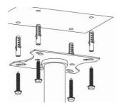
This bracket is designed to be modular, and interchange with brackets that use the same  $2^{\prime\prime}$  (51mm) pole standard.
