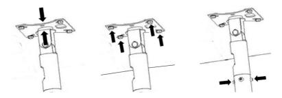
5. Attach projector to the spider/bottom yoke fitting to the projector, and attach all to the pole.
